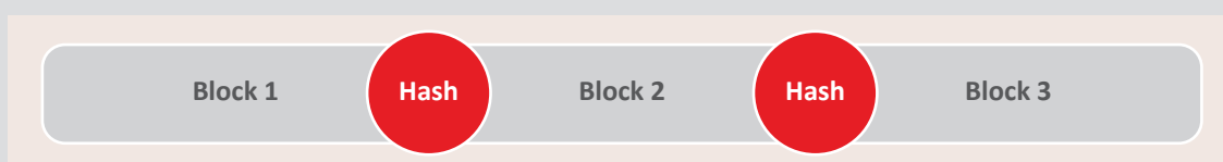
Figure 2a: Blocks of Data Forming a Blockchain in a blockchain, data are grouped into blocks that are then “linked” together using digital signatures on cryptographic hashes.
